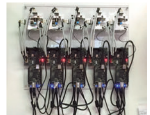
Testing one of the first batches of Formlabs-built galvanometers
